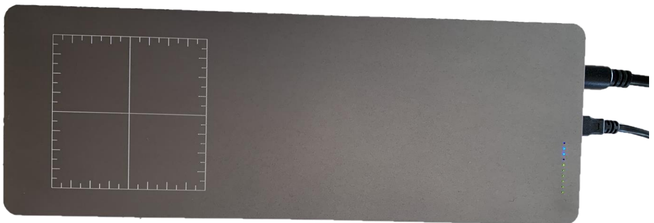
HallinSight® 32X32 pixels sensor array
