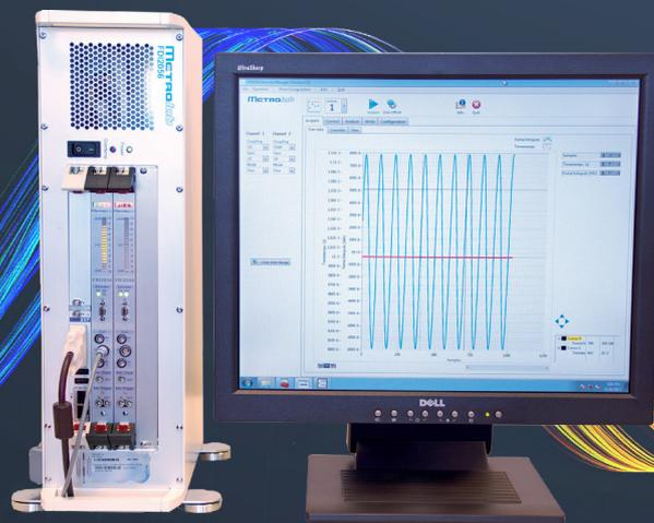
The Fast Digital Integrator FDI2056 is the world's fastest and most sensitive voltage integrator. Plug in a sense coil, and for the first time it is possible - even easy - to measure fast, low-level magnetic field disturbances such as eddy currents in a switched magnet.
