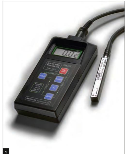
sensor, measures a field component in the semiconductor plane (Figure 2). Combining a planar with two vertical Hall sensors on the same chip results in an integrated three-axis Hall sensor. Compared with a traditional three-axis probe consisting of three discrete sensors glued to a
