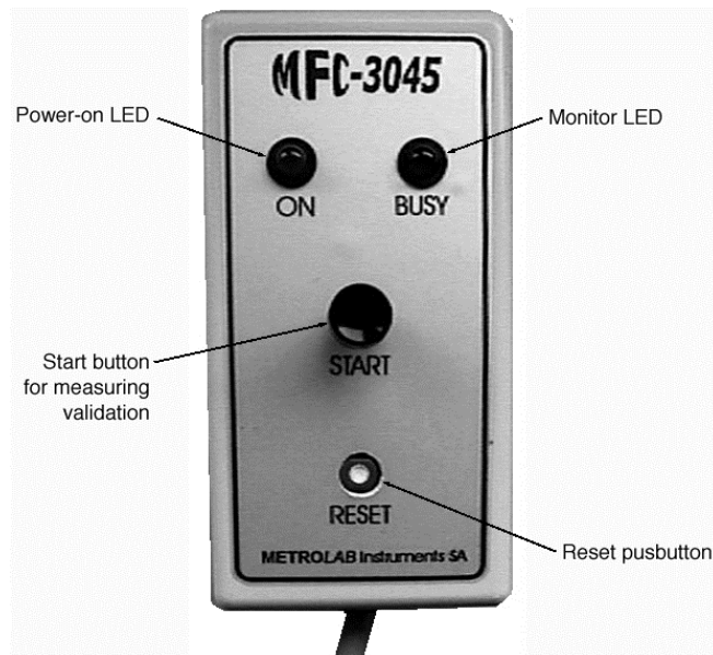
Figure 10 : View of the Remote Control box and its commands
