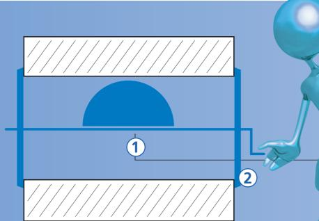
The measurement of the magnetic field is based on the NMR CW (Continuous Wave) principle, with frequency modulation. Fields from 0.2 to 7 T are measured with a relative precision better than 0.2 ppm. The stability and resolution of the system allow superconducting decay monitoring. The user can modify all measurement parameters.
